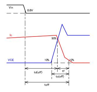
Fig.2-2: Operation sequence of Over current protection
