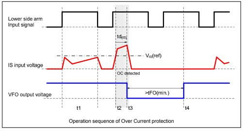
t1: IS input voltage does not exceed  $V_{IS}$ (ref), while the collector current of the lower side IGBT is under the normal operation.
