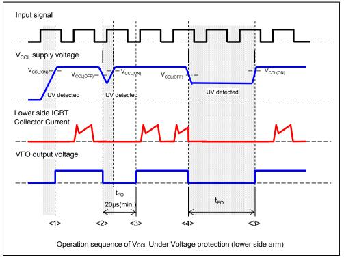
When VCCL is under 4V, UV and fault output are not activated.
